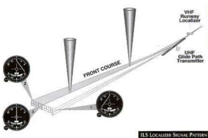
Figure 6 – ILS LOCALIZER SIGNAL PATTERN
