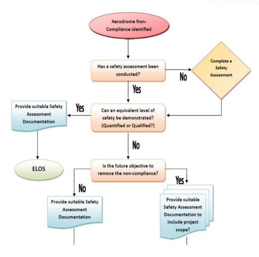
The flow chart provides an overview of where non-compliance should be placed. Based on the documentation submitted, it will enable GCAA place non-compliance on the Authority's regular oversight program until completed.
