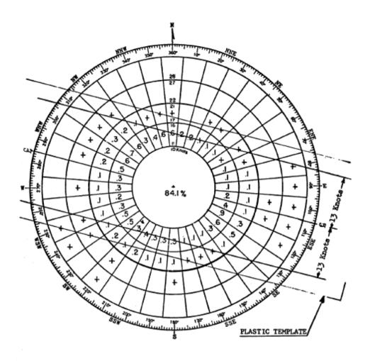
A runway oriented 105 – 285 (true north) would have 2.72% of the winds exceeding the design crosswind/crosswind component of 13 knots
