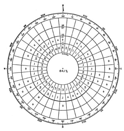
Figure A2-3. Completed windrose using A2-2 data
