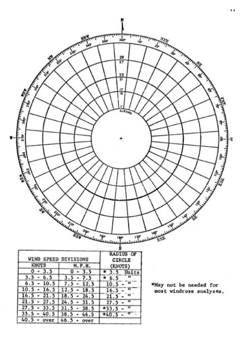
Figure A2-1. Windrose blank showing direction and divisions
