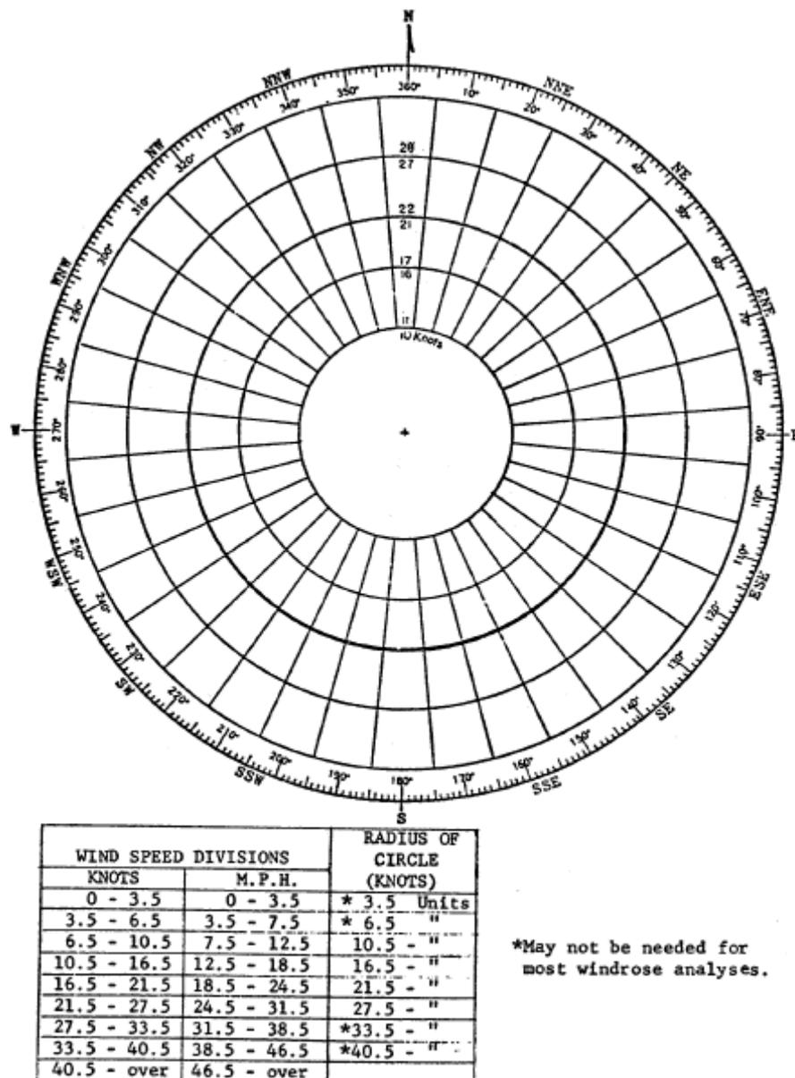
Figure A2-1. Windrose blank showing direction and divisions
