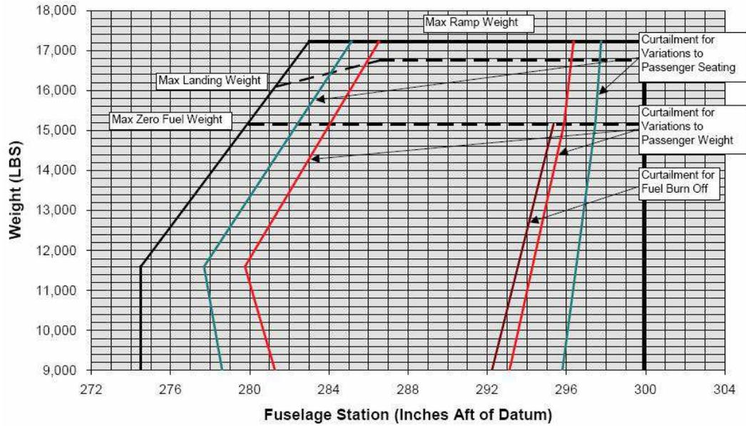
To expand the operational loading envelope, an operator could choose to use the actual seating location of passengers in the cabin and reduce the curtailment for variations in passenger seating. Figure A-17 below shows the expansion of the operational loading envelope
