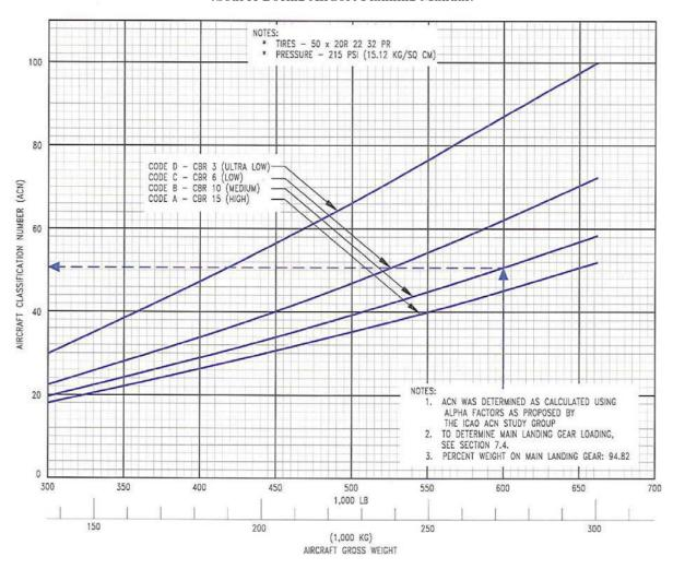
The common form of presenting the ACN values for a known operating tyre pressure is to tabulate the values calculated for each of the four standard subgrade strengths for the aircraft at Maximum Take-off Weight (MTOW) and Operating Weight Empty (OWE).
