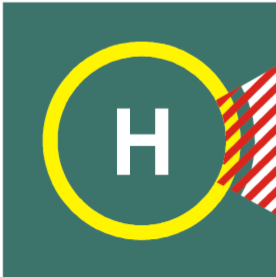
Figure 5-7. Helideck prohibited landing sector marking
