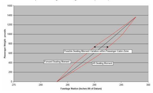
1) **Determining the most adverse loading.** It is important that an operator examine the above results (from Figures A-4 through A-15) for each zone and determine which loading scenario results in the greatest difference in moments.
