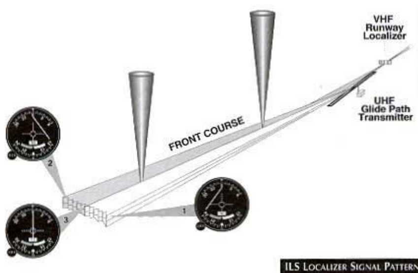
Figure 6 – ILS LOCALIZER SIGNAL PATTERN
