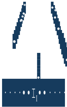
SIMPLE APPROACH AND RUNWAY LIGHTING SYSTEM
